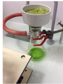
Use a Buchner filter to filter the solvents and avocado flesh.
